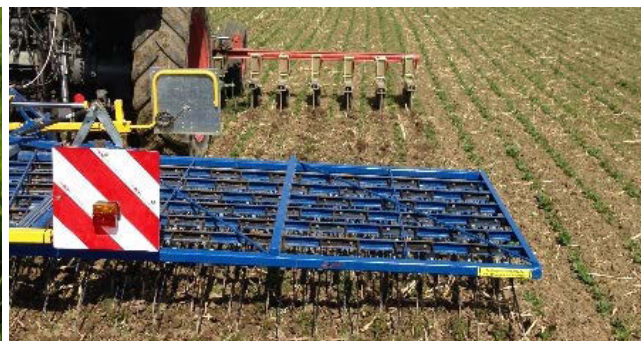
Picture 1: Wide row, here in barley (Photo: Hansueli Dierauer, FiBL). Picture 2: Combination of a 6 m hoe (front) with a harrow (back), here in soya (Photo: Ueli Weidmann, FiBL).
