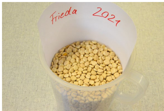
The samples from different locations of a batch are mixed to form an aggregate sample (well homogenised).
