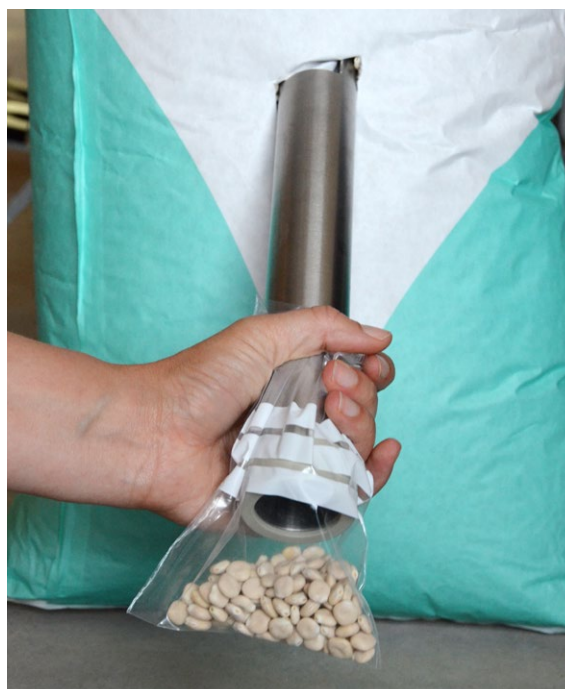
The sample spear can also be used to take individual samples from the lower layers of a bag.
