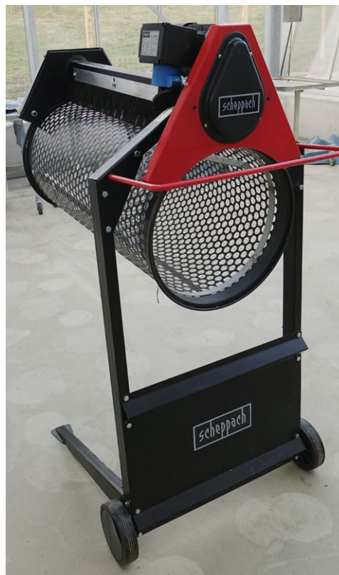
Rotary screen for sieving the compost or the final substrate
