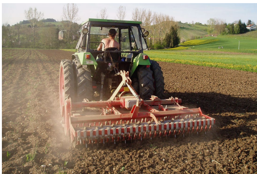
In a first passage, the field can be refined and levelled with a power harrow.
