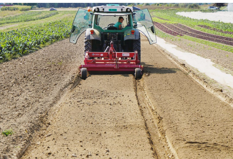
Final seedbed preparation is commonly managed with a rotavator. A too fine tilth can have negative impacts on soil structure and soil biology.
