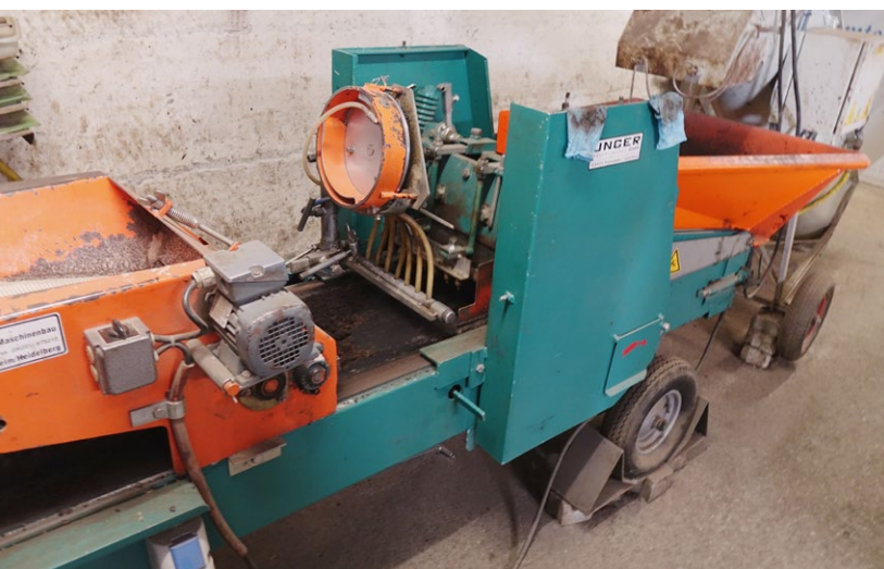
Complete seedling line with a pneumatic seeder
