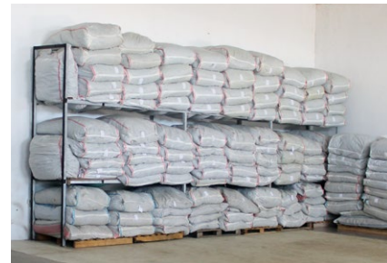
These bags are stored too close to the wall. This can cause moisture to accumulate between the wall and the bags.
