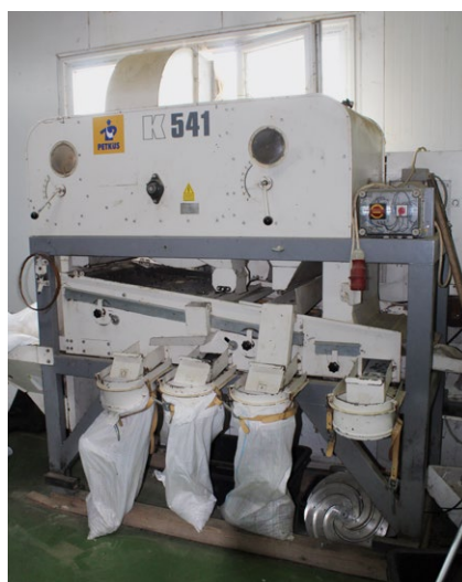
Screen separator to remove fine particles and sort the dried product into different categories.
