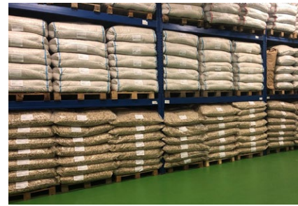
Storage of the sacks on wooden pallets ensures sufficient distance of the crop from the ground.
