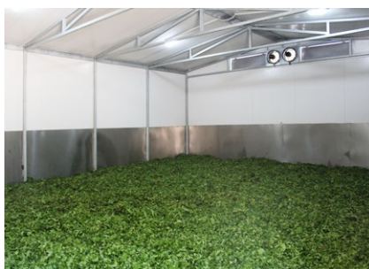
Container dryer filled with fresh MAPs
