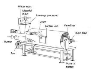
Figure 2. System schematic diagram of the drum roaster installed at Stadlhuber Agrar.
