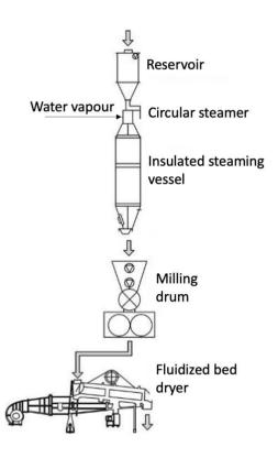
Figure 4. Layout of the hydrothermal treatment system with circular steamer, steaming vessel, milling drum and fluidised bed dryer.
