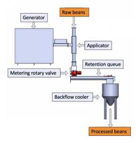
Figure 5. Model for the Florapower continuous oscillation heater
