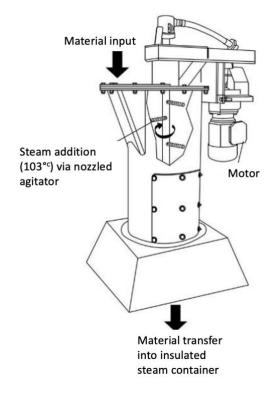
Figure 3. System schematic diagram of the circular steamer.
