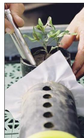
*This testing system makes it possible to quantify nutrient intake through mycorrhizal hyphae.*
