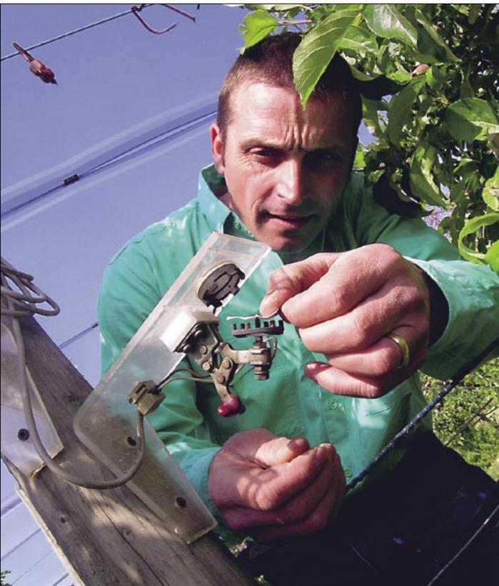
*The weather station requires careful maintenance in order to deliver reliable data. The photograph shows Christophe Suter exchanging a piece of blotting paper which simulates leaf wetness.*
