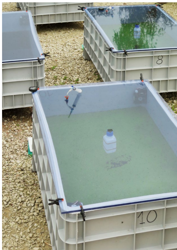
Temperature measurements and acid trap for measuring ammonia emissions in a duckweed pallet box with transparent lid.
