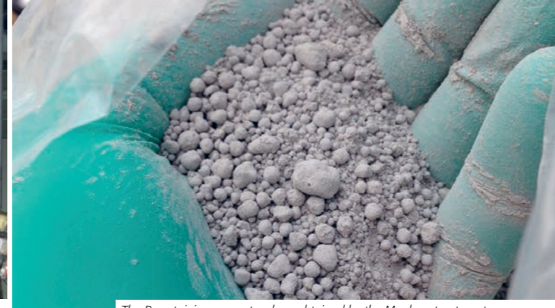
The P containing converter slags obtained by the Mephrec treatment
