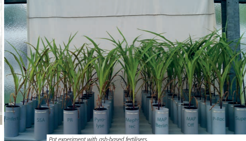
Pot experiment with ash-based fertilizers.
