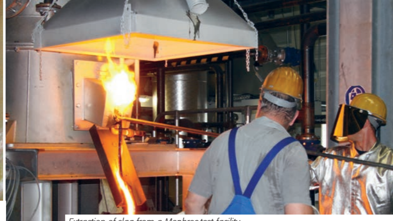
Extraction of slag from a Mephrec-test facility.
