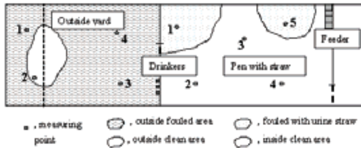
Figure 1: Measuring points and fouled areas in pens of 45-kg fatteners on farm 1.
