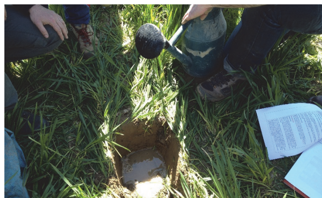
Figure 2: Mustard solution is poured into the hole and the infiltration is measured. Photo: D. Antichi
