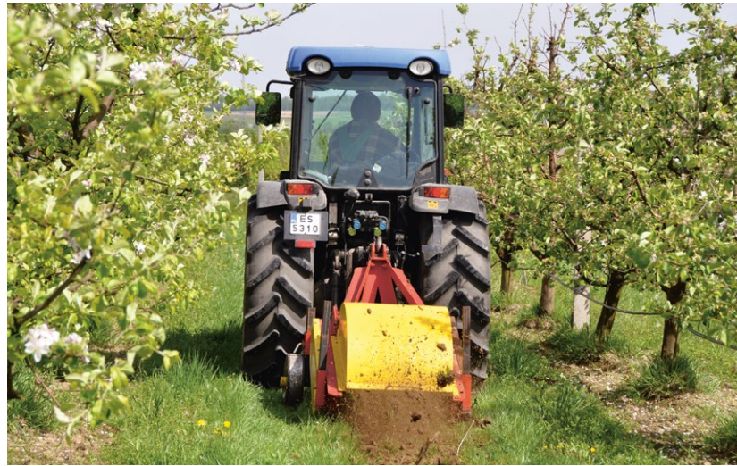
The recommended width for flower strips is equal to the inner distance between the tractor wheels plus 10 cm, resulting in a 5 to 10 cm overlap into the tractor track at each wheel. Flower strip width also depends on the available machinery for soil preparation and mulching.
