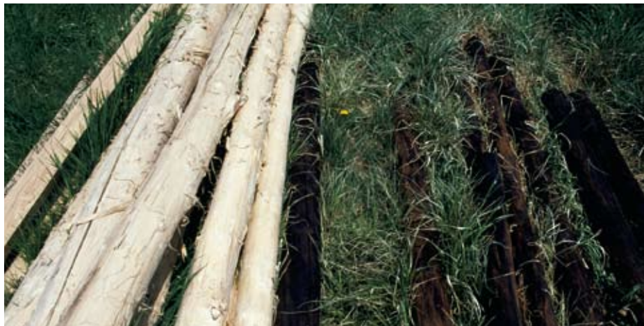
Unlike creosote timber (right), non-impregnated robinia poles (left) do not cause any plant burns (pay attention to the growth of grass between the poles).
