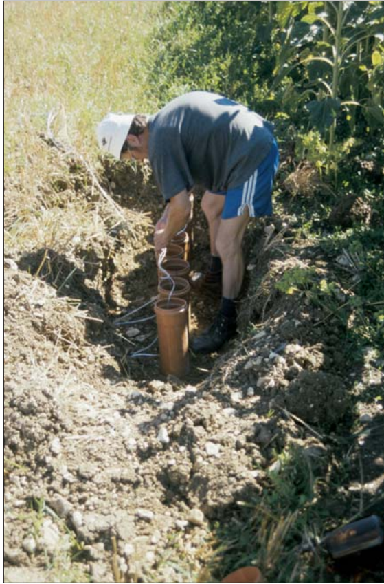
The gravely soils in the Klettgau region are readily permeable and therefore greatly at risk of wash-out. Monitoring performance: The measures adopted are checked by means of suction cups.
